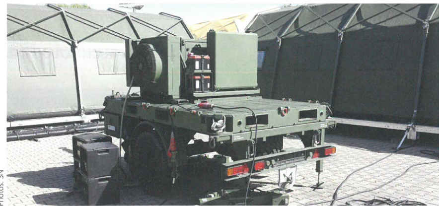
Air-transportable generator trailer (Grünenfelder) configured by M. Schall GmbH for EU Battlegroup field camps. Two such generators can provide electricity for a large protected tent module.
