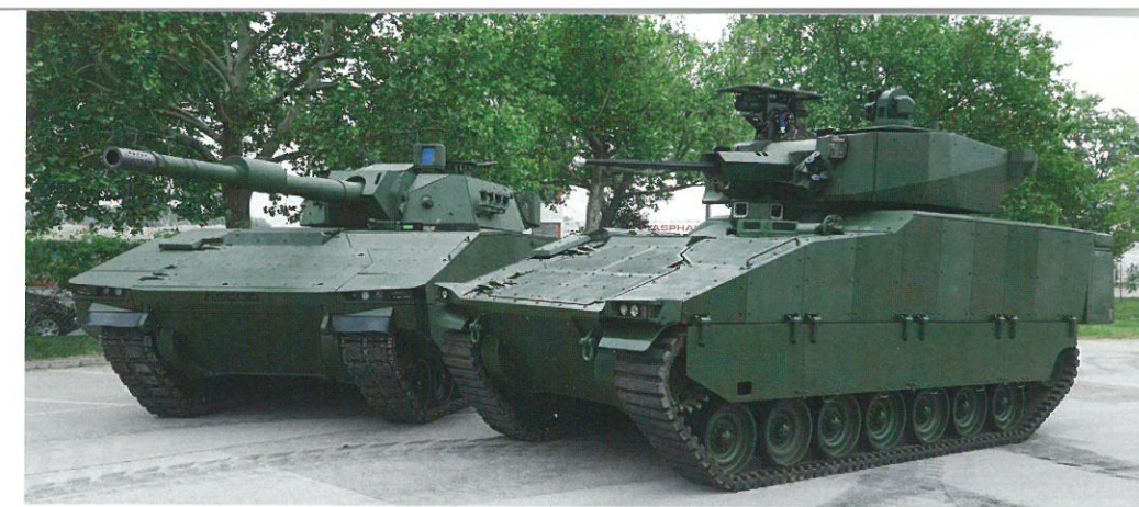
ASCOD MMBT (left) and the new ASCOD IFV with the UT30MK2 turret on display at the outdoor area of GDELS-Steyr in Vienna, Austria
